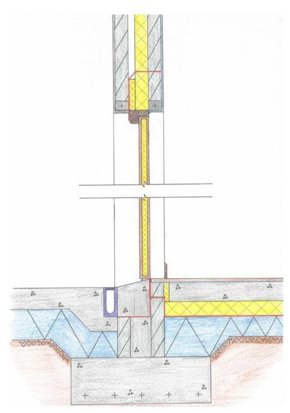
The Door Threshold (where the bottom of the door meets the finished floor/cill) must ensure that it is able to resist wind-driven rain.
