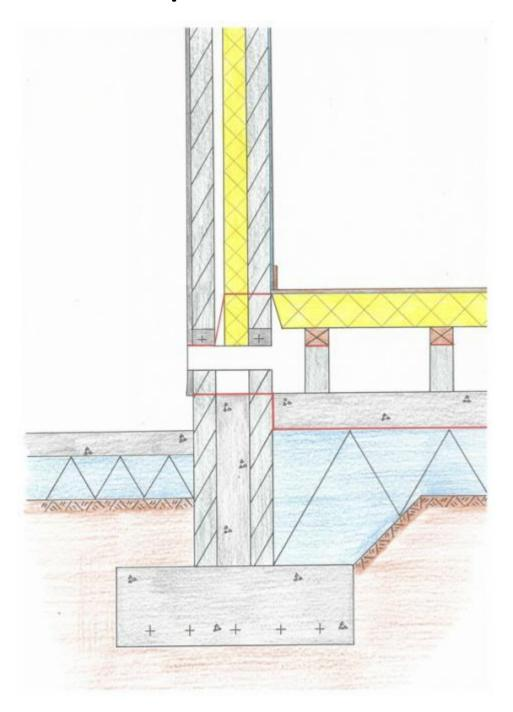
Suspended Timber Ground Floors consist of the finished timber floorboards being attached to floor joists, which are suspended above the subfloor of the foundation.
