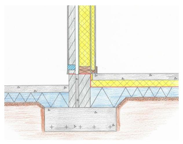
Timber Frame Construction is quite similar to concrete cavity wall construction as the outer leaf remains as masonry, a 50mm cavity is installed, with the only difference being a timber frame internal leaf.
