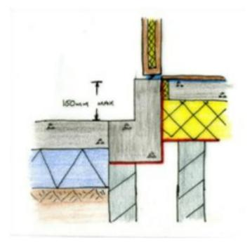
There is also a stepped alternative for the threshold detail.
