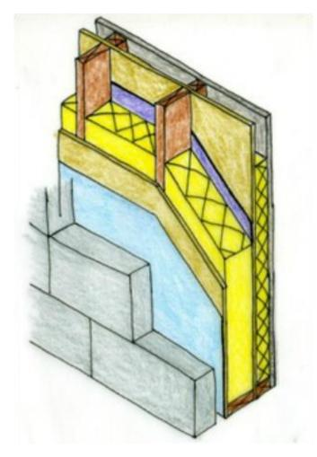
The combined protection provided by the vapour barrier (internally) and the breather membrane (externally) ensures the timber inner leaf remains dry at all times.
