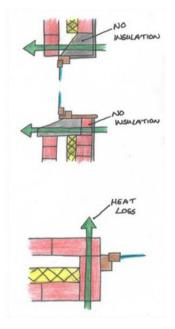
To prevent this, the window head and cill must show correct installation of insulation and damp proof courses.
