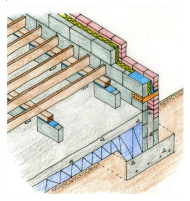
To ensure that the floor is thermally insulated, either rigid or blanket insulation is placed between the floor joists.
