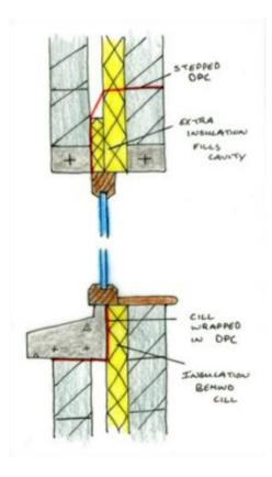
The horizontal section of the window jamb must also incorporate correct insulation and damp proof courses to prevent cold bridging.
