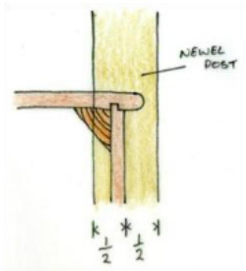
The handrail is parallel to the string and is fitted into the newel posts. The handrail and the balusters form the balustrade which provides protection on the open side of the stairs.
