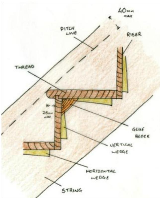
The staircase itself consists of two strings, in which the steps are housed into to ensure a secure and safe unit.
