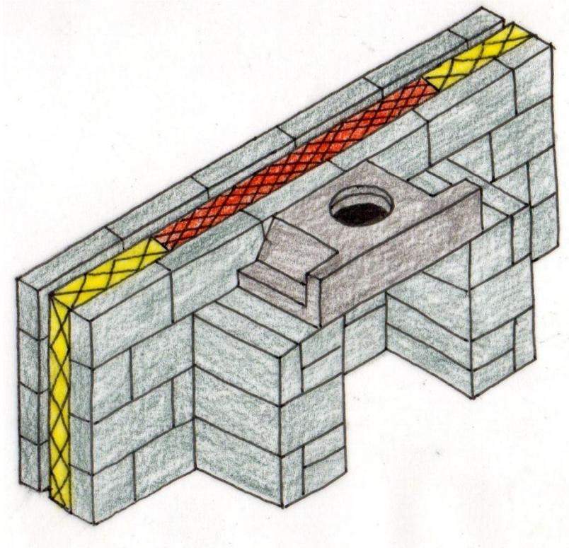
*A 500mm minimum hearth must extend from the fireplace to ensure safety from heated elements from the fire.*
