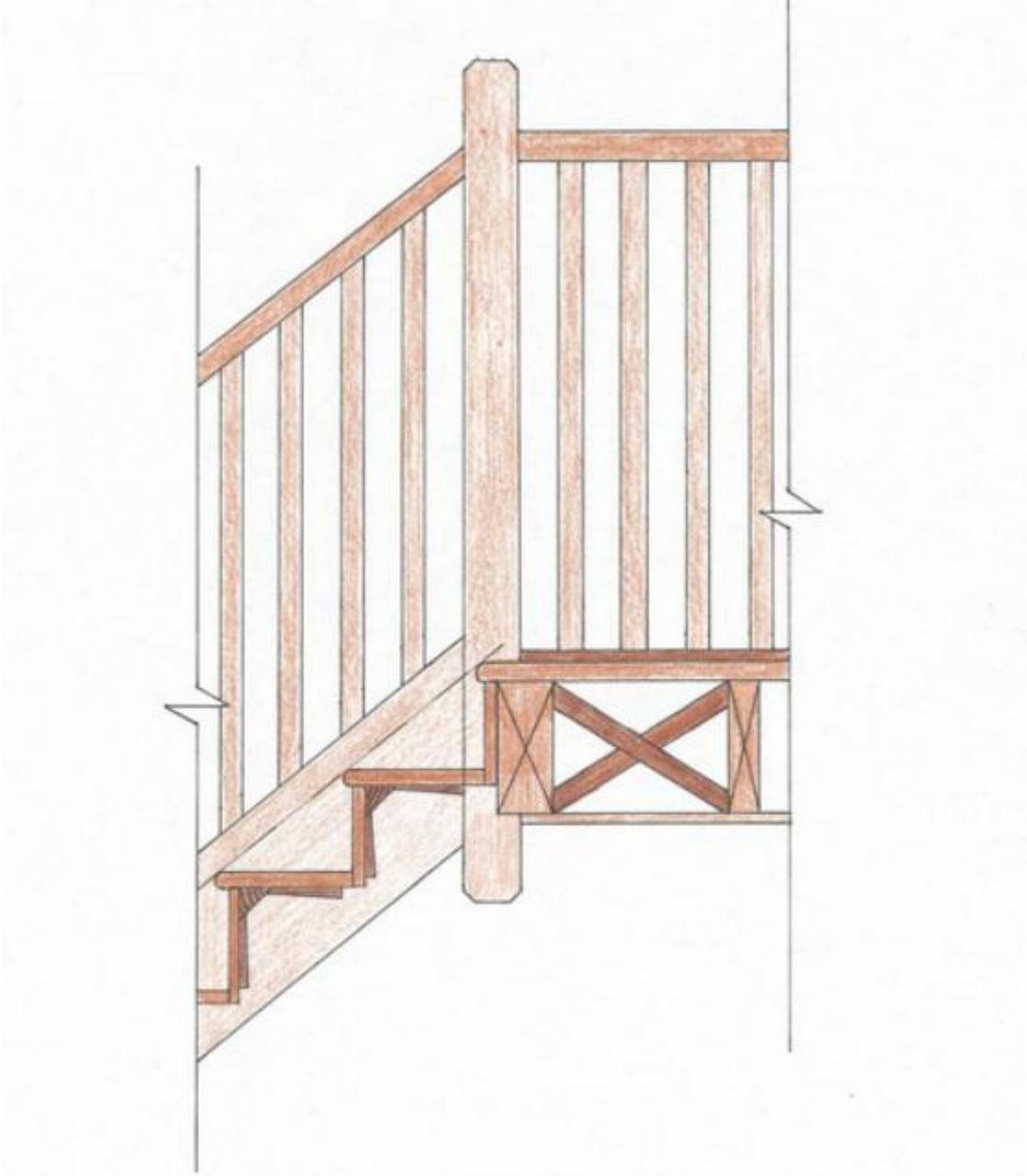
*The top of the stairs detail displays the joining of the staircase with the landing of the upper floor.*
