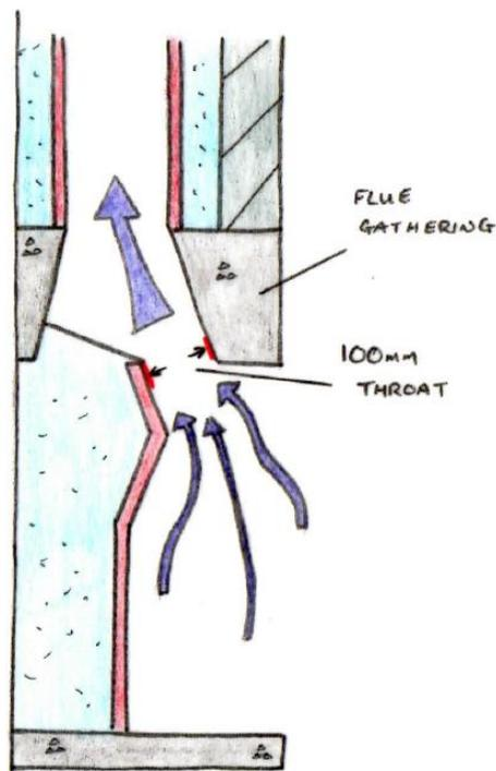
A precast concrete flue gathering is used to ensure that a 100mm throat is in place. A variation in the size of the throat will have a significant impact on the performance of the fireplace. (It creates a sufficient 'pull' for the smoke of the fire)
