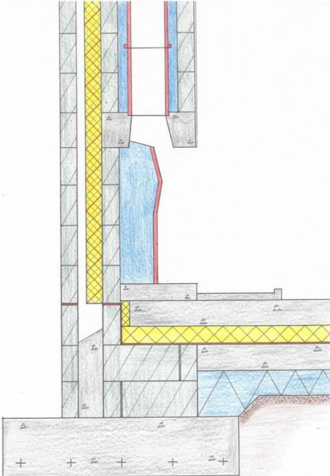
*The foundation must be extended under the fireplace to ensure that the extra loads of the fireplace and chimney are catered for.*
