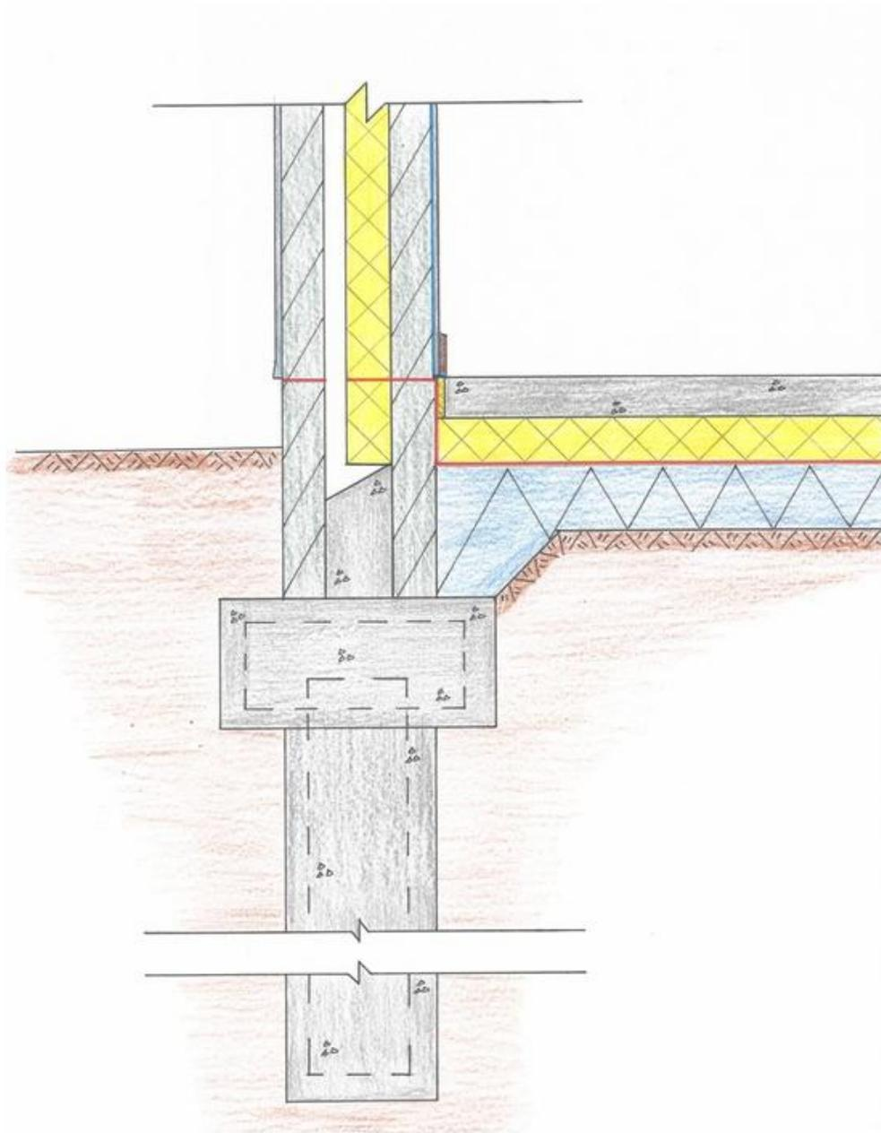
*A pile is a column of concrete that extends downward deep into the soil.*
