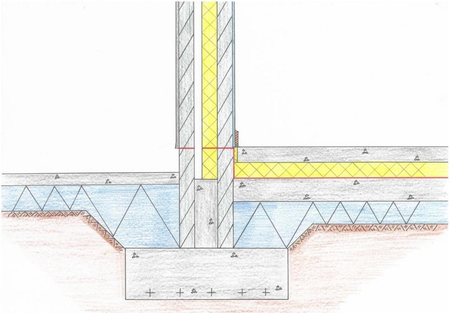
*The size and position of a concrete strip foundation is directly related to the overall width of the wall.*
