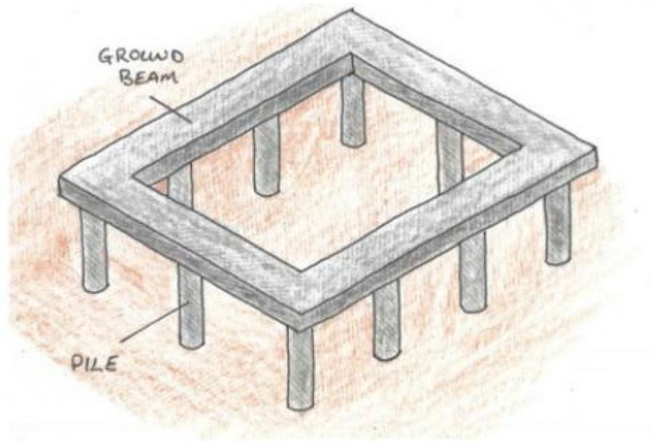
*One method of construction is to drive precast piles into the soil using specialised percussion drivers. The other method requires the drilling of a pile hole in the soil, which is then poured with concrete and reinforced with steel.*
