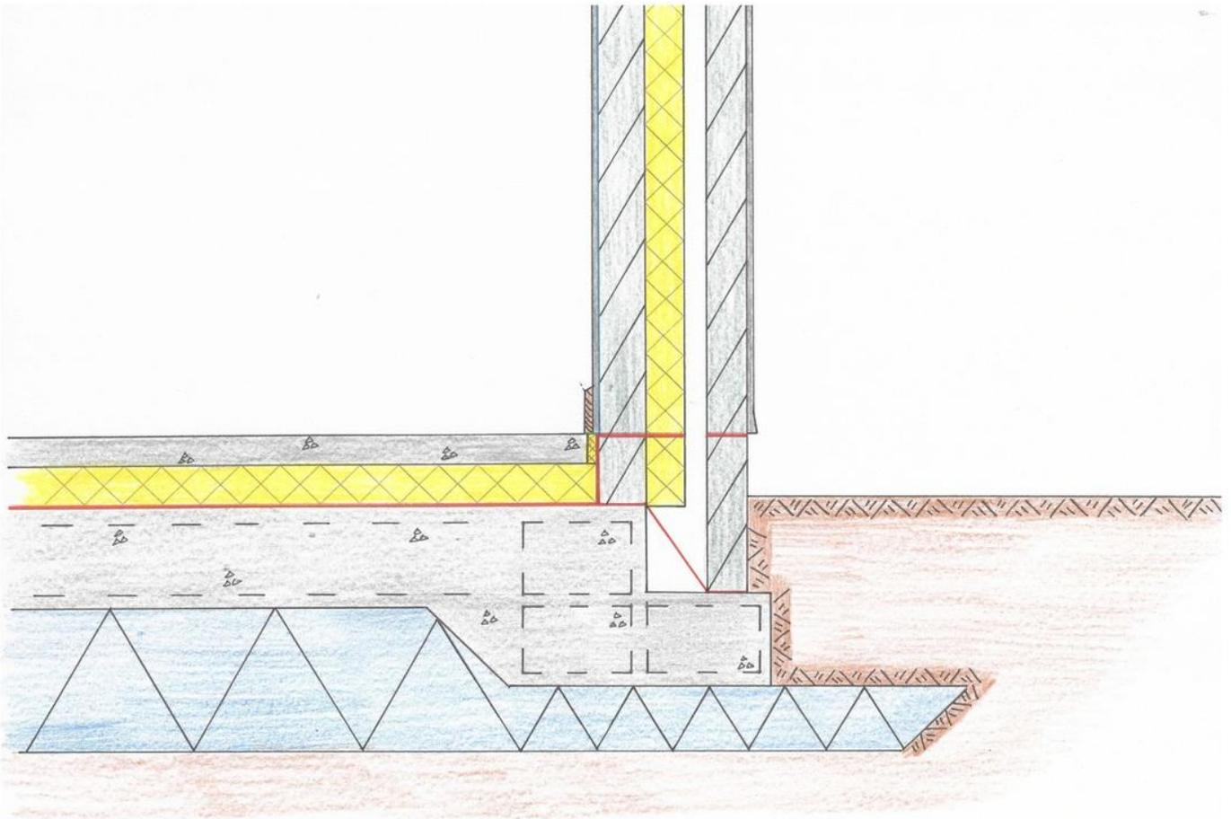
*The concrete raft is supported on a compacted hardcore base which extends out past the edge of the raft.*
