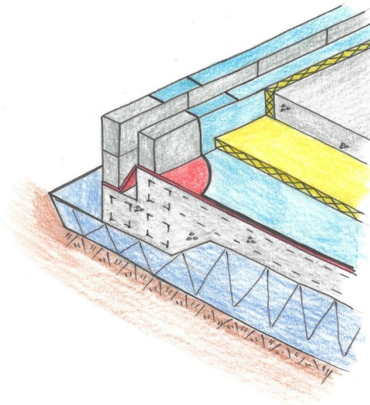
*100mm of rigid insulation is installed below the finished floor to ensure that there is no heat lost through the foundation.*
