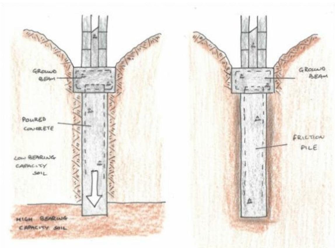
*Once the piles are complete, the ground beam can be created. This is the surface of which the walls of the dwelling can be built.*
