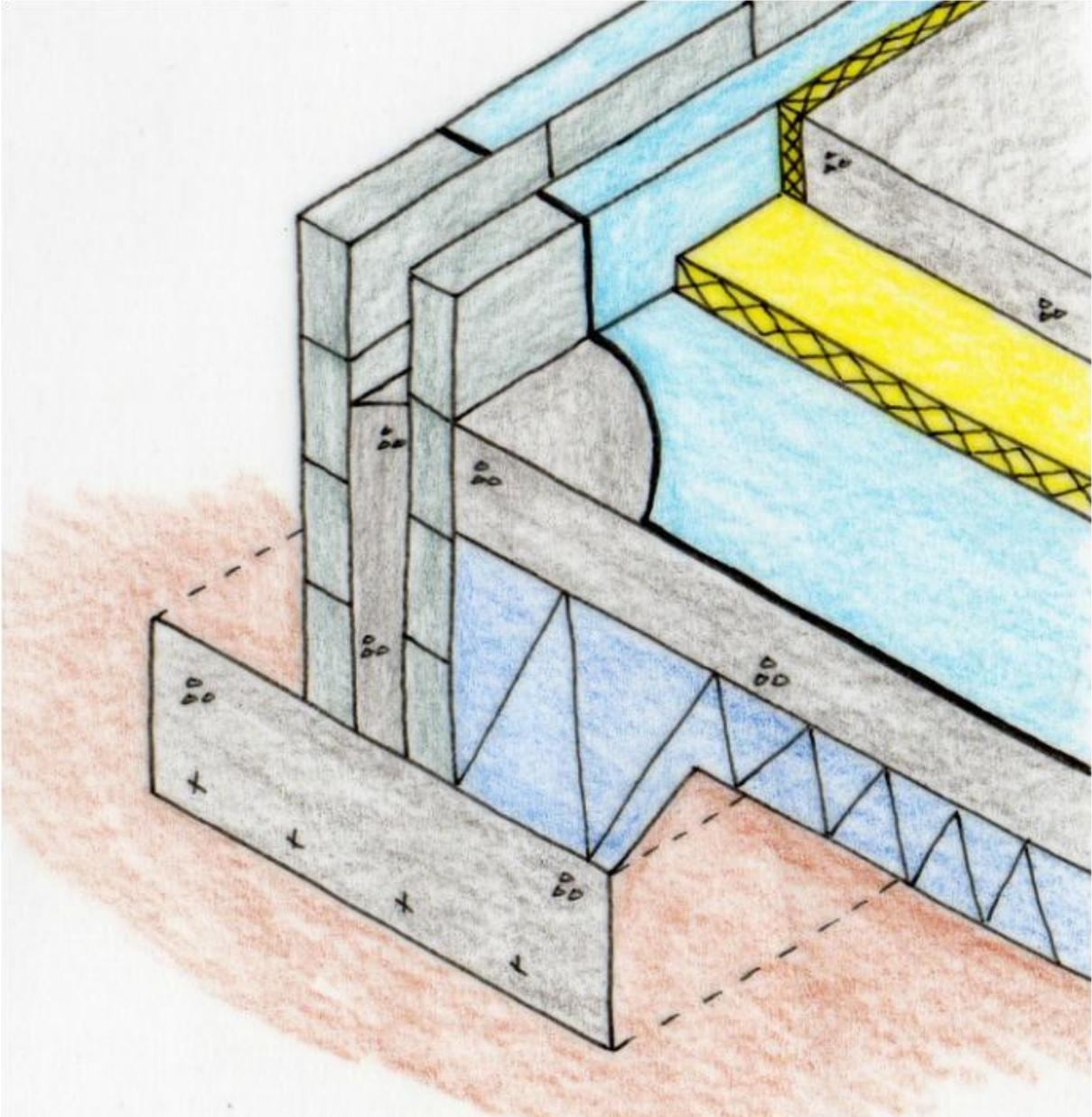
*100mm of rigid insulation is installed below the finished floor to ensure that there is no heat lost through the foundation.*
